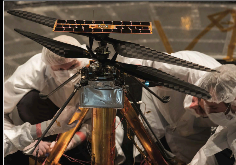
When NASA's Perseverance rover lands on February 18, 2021, it will be carrying a passenger onboard: the first helicopter ever designed to fly in the thin Martian air.
